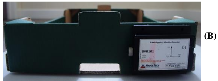
Figure 6.10: Vibration logger SVR101 (A) and the method of logger attachment onto the corrugated fibreboard box during measurement (B). Source: Chaiwong (2015).
