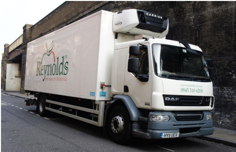
Figure 6.1: A refrigerated truck of 18 tonnes on the London route. Source: Chaiwong (2015).
