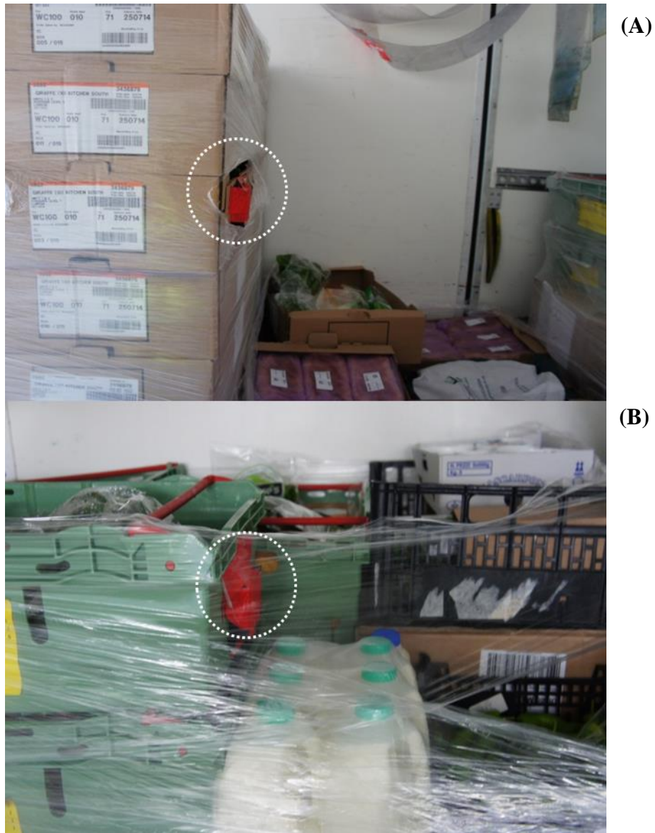
Figure 6.9: The attached vibration logger on the corrugated fibreboard box (A) or plastic crate (B). Source: Chaiwong (2015).
