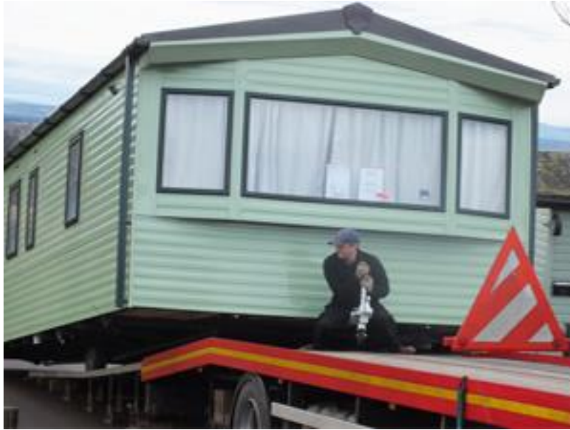
Figure 30: A static caravan being unloaded from a caravan transporter of Northlodge Transport. As the caravan is slowly winched down the 'beaver-tail' and 'skids', the driver or his assistant keeps the caravan in line by guiding the jockey wheel. The winch is operated remotely with a control pad linked by cable to the winch motor; for smaller units the driver can manage the whole loading and unloading operation if required.
