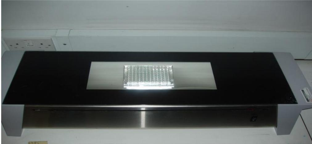
**Figure 4.3. LumiSource™ (PCI Biotech) lamp used for irradiation.**
