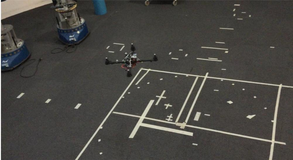
FIGURE 3.28: Individual Quadrotor in Path Tracking Flight
