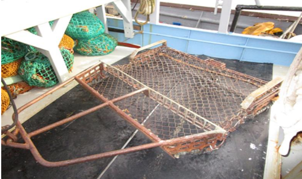
Figure 4 Modified Ladder Dredge used by oystermen in the Essex Estuaries for oyster cultivation. note, the silver bar and the silver skis are the only area of the dredge in contact with the sea bed.
