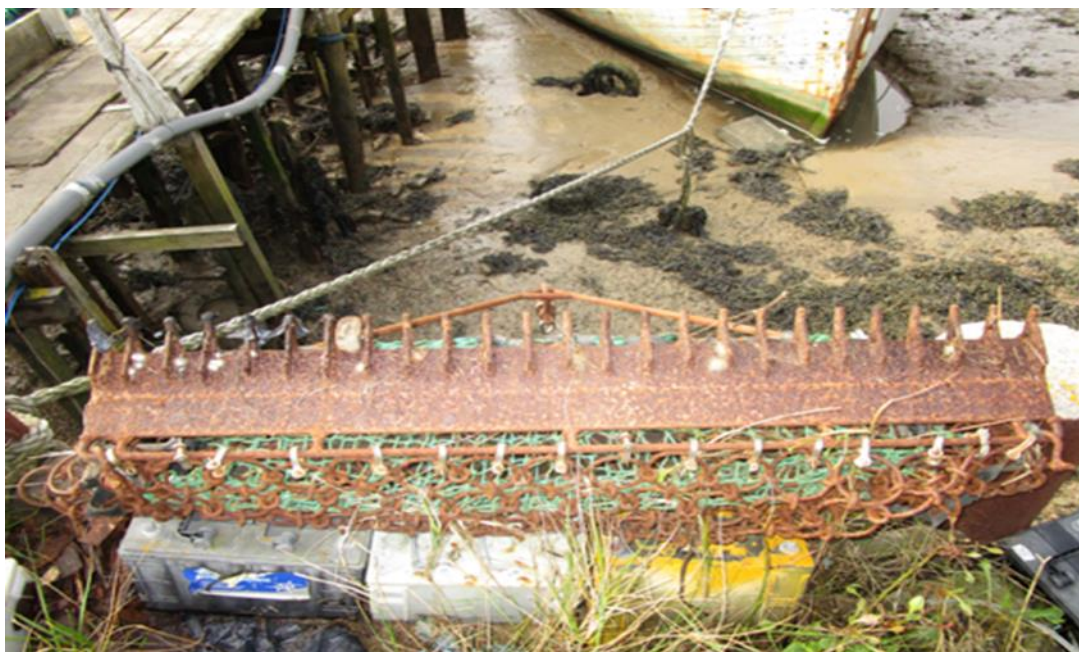
Figure 5 An example of a toothed oyster dredge, now redundant in oyster cultivation practice in the Essex Estuaries in favour of less invasive ladder dredge (see figure 4)
