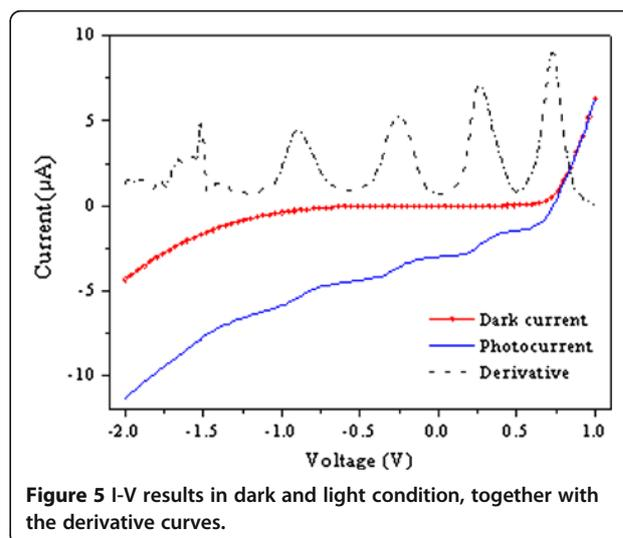
The photocurrent in Figure 5 has two components; the thermionic current which increases monotonically with applied bias and the oscillatory component which is the resonant tunnelling current [26]. In order to show clearly the oscillatory component, we took the first derivative of the photocurrent. The peak current values correspond to the resonant conditions in the wells adjacent to the anode similar to those as described in references [26,28].
