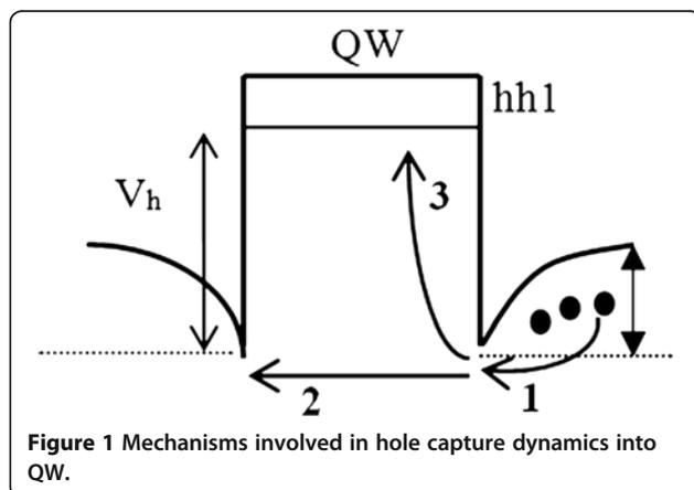
**Figure 1** Mechanisms involved in hole capture dynamics into QW.
