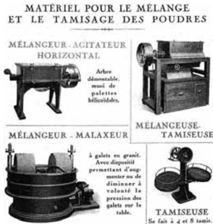
Equipment for Mixing and Sieving Powder. Savy Jeanjean catalogue, 1906.
