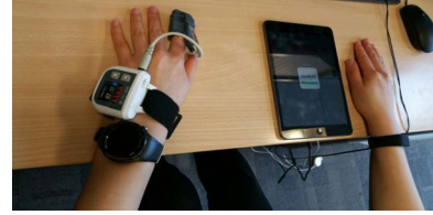
Fig. 1. A subject wearing the Wavelet Health wristband on the right wrist; the Huawei watch series 2 and a PC-68B pulse oximeter on the left hand.
