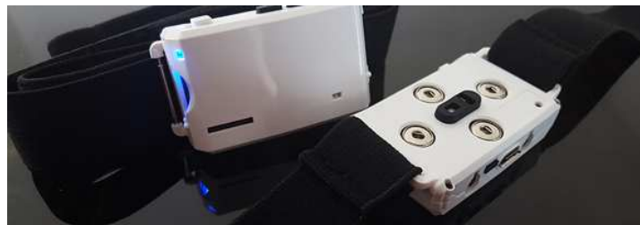
Figure 1.6. The front and back side of Hypnodyne ZMax. On the back side the photoplethmograph (PPG) sensor can be seen in the middle, encased in a soft plastic cover. In addition, the for clip-on inserts for ZMax's proprietary disposable electrode patch can be seen surrounding the PPG sensor.
