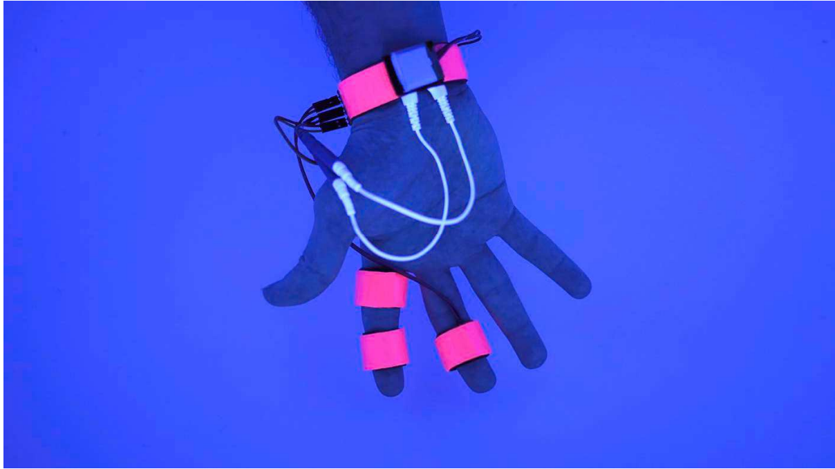
Figure 1.5. Dormio hand-worn device developed by MIT. Dormio includes an accelerometer, wrist electromyogram (EMG) sensor and photoplethmograph (PPG) finger sensor to measure heart-rate galvanic skin response (GSR) sensors located at the fingers. Image taken from https://www.media.mit.edu/projects/sleep-creativity/overview
