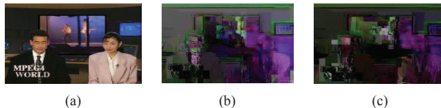
Fig. 4. Impact of keys on video perception of the News sequence encoded with 90 frames (I+P+B) and QP 24. (a) Frame # 41 [Y=42.29, U=45.15, V=46.33] dB, (b) e_k change by 1 bit [Y=11.34, U=19.87, V=24.78] dB, and (c) e_k change by 2 bits [Y=11.37, U=19.79, V=24.70] dB.
