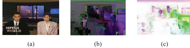
Fig. 3. Impact of replacement attack on the News sequence encoded with 90 frames (I+P+B) and QP 24. (a) Frame # 41 [Y=42.29, U=45.15, V=46.33] dB. (b) Proposed SE [Y=11.35, U=19.92, V=24.32] dB. (c) Replacement attack [Y=3.94, U=17.58, V=19.01] dB.
