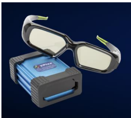
Figure 2.1: 3DPixx system. Image taken from https://vpixx.com/products/3dpixx/ showing the infrared (IR) emitter and 120Hz LCD glasses used to synchronise 3D stimuli on screen with the glasses.
