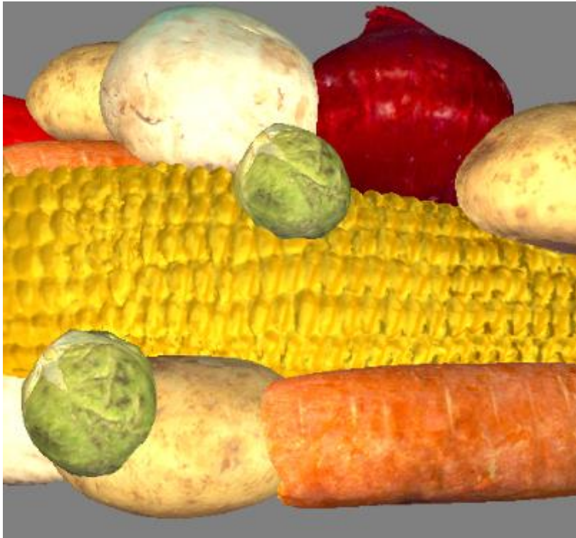
Figure 2.2: Results of scanning. Showing a selection of naturalistic fruit and vegetable 3D models created using the scanners listed above. The sweetcorn was scanned using the Artec Spider, and the remaining models were scanned on the NextEngine scanner using the turntable.
