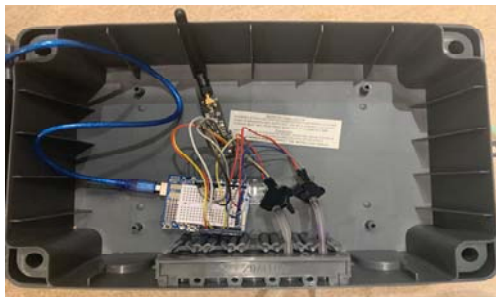
Figure 5 Transmitter End of the system
