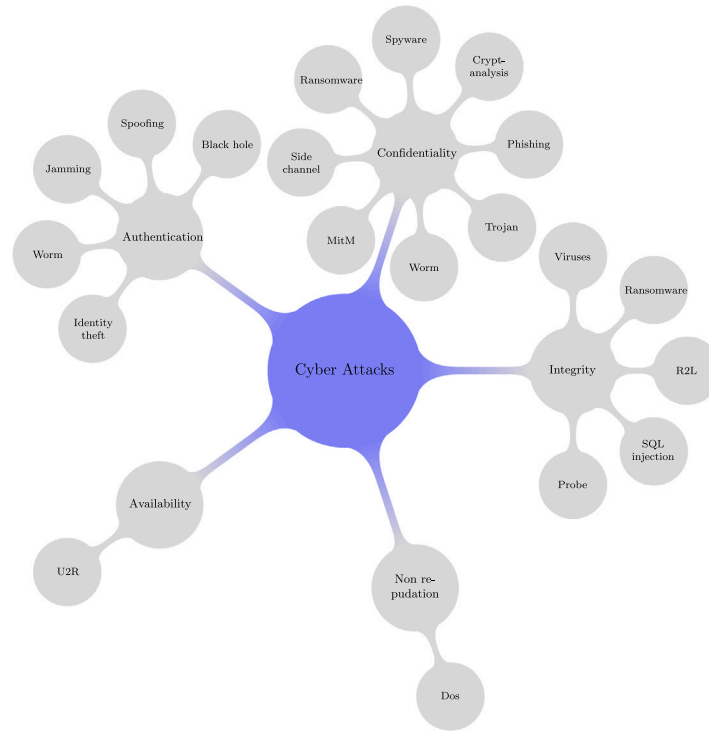
Fig. 3. This taxonomy classifies attacks according to security services. The most common attacks used to violate these services are display. Man in the Middle attack (MitM), Denial of Service attack (DoS), Root to Local attack (R2L), User to Root attack (U2R), Probe (Probing attacks), and Structure Query Language Injection attack (SQL injection).
