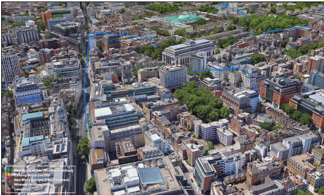
Figure 9.1: Final modelling results imported and visualised in Google Earth ©2023 Google. (Central London, D-band 159.125 GHz transport, O-RAN option 7.2x fronthaul, roof top and street level infrastructure, cell density 200 m.)
