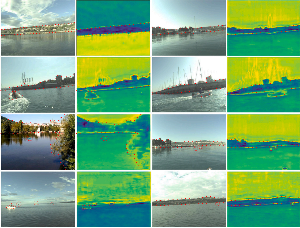
Fig. 8. The visualization of navigation scenario images paired with their corresponding C-TEF semantic weight W_1 , as shown in Fig. 6. In this visualization, the red dots denote boundaries with increased weight values, while red dashed lines delineate areas with small water surface targets. It is observed that, in various scenarios, elevated weights are not only assigned to boundaries but also to regions with small water surface targets, demonstrating a heightened attention of the semantic weights on these challenging areas for classification purposes.
