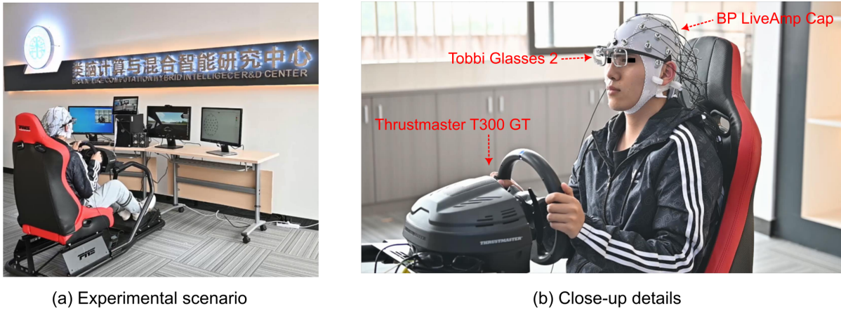
Fig. 1. The system of multimodal driving fatigue detection. (a) experimental scenario. (b) a subject wearing an EEG cap and a pair of Tobbi Glasses was driving a simulated vehicle in the simulation platform.
