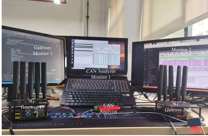
Fig. 10 The experimental platform used for testing the integration of 5G and CAN networks
