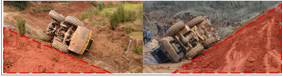
Fig. 1. Typical unstable driving accidents of ACVs.
