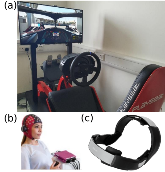
Figure 1. Main hardware items of the experimental setup. (a) Driving simulator (b) ANT neuro eego EEG system (c) PlatoScience PlatoWork tDCS system.
