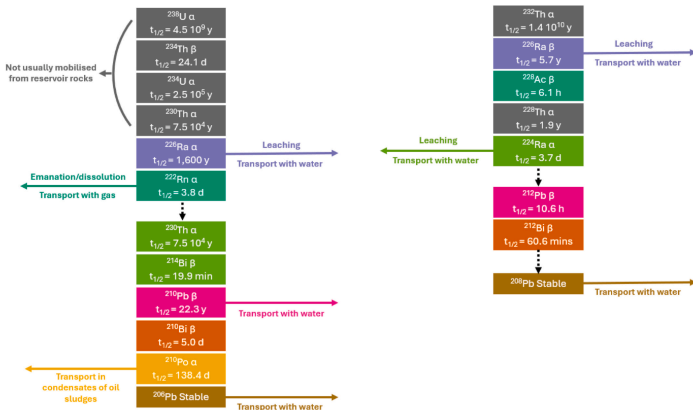
Fig. 2. Transport of (a) 238 U and (b) 232 Th and their key decay products during O&G production (adapted from Jonkers et al., 1997; IAEA, 2003). Note: Short lived radioelements (i.e. t_{1/2} < 5 min) are not represented in this illustration.
