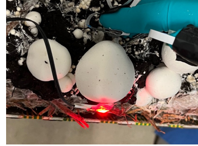
Fig. 3: Experimental configuration for root stiffness characterization during bending action with a Touchence Shokac Chip force sensor attached on the finger that will perform the action, and the Phasespace tracker led for measuring the total displacement.
