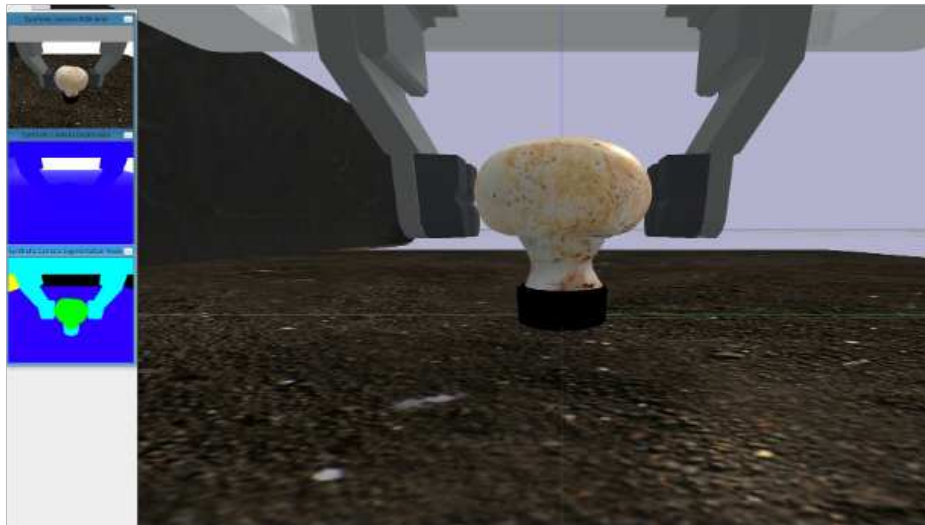
Figure 3.4 The PyBullet debug GUI view of the simulation framework for mushroom harvesting.
