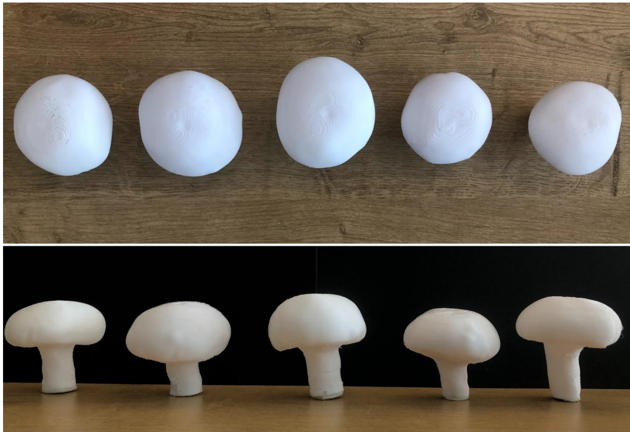
Figure 5.2 Top- and side-view of the five mushroom models used in the picking experiments.
