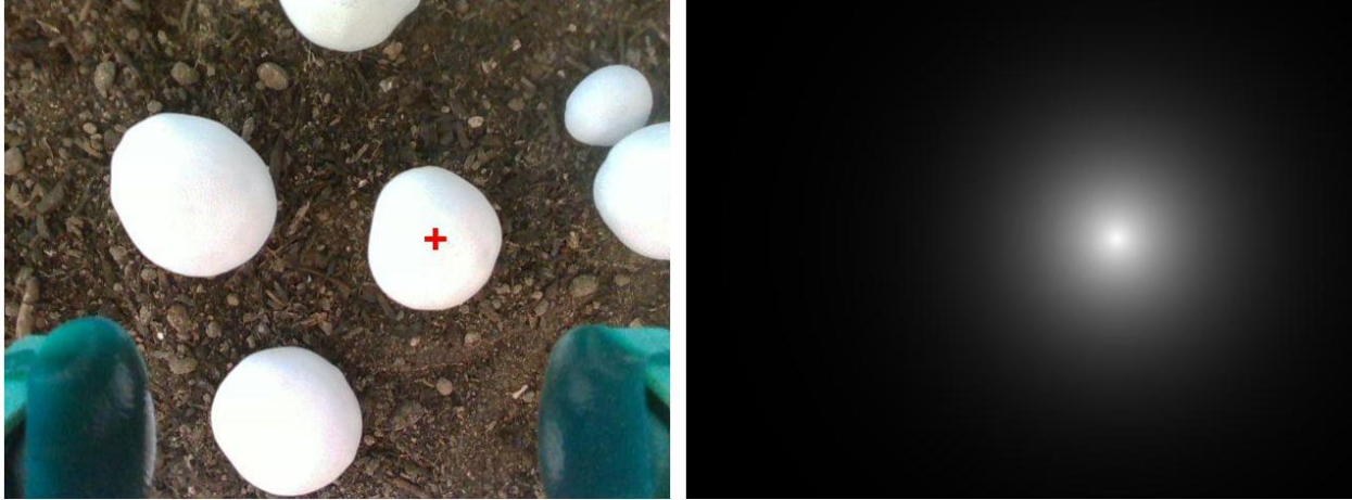
Figure 7.5 Indicative example of determining a target mushroom. Right: Target pixel is painted on the image. Left: Extra image channel carrying an inverse modulated distance map as described in eq. (7.9).
