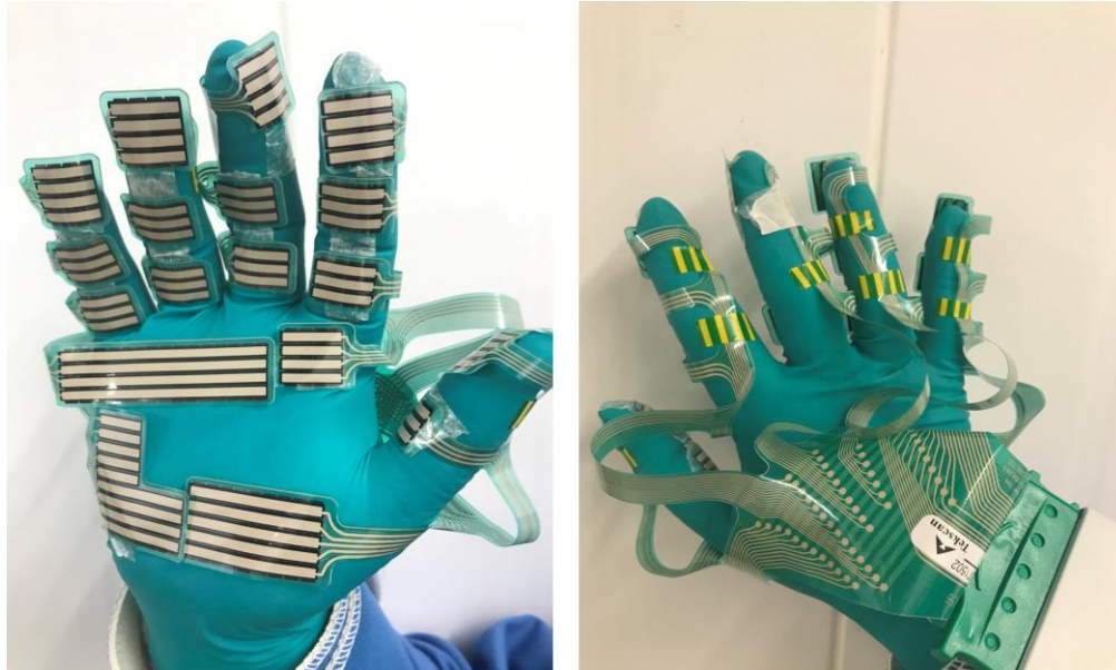
Figure 3.5. Tekscan Grip System sensing elements mounted on the mushroom picker's gloves.
