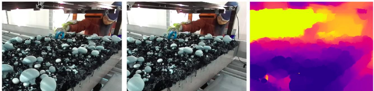
Figure 3.11 RGB-D camera 2: Left Image, Right Image and Depth Array
