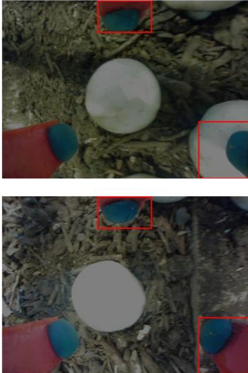
Figure 6.11 Annotated screenshots during trained agent (vq-rec) episode rollouts: (a) the bottom left right finger is significantly displaced due to collision with a nearby mushroom, (b) the top finger is moderately displaced due to hysteresis.
