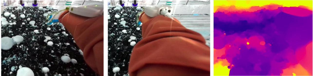
Figure 3.10 RGB-D camera 1: Left Image, Right Image and Depth Array
