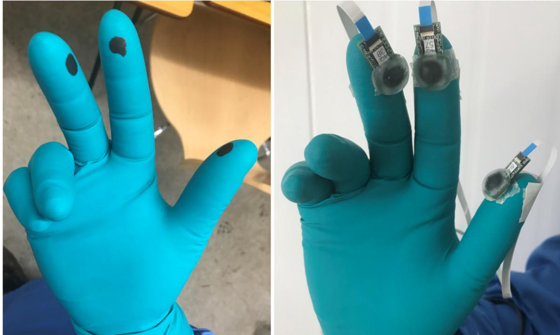
Figure 3.7 Force sensors mounted on the expert picker gloves.
