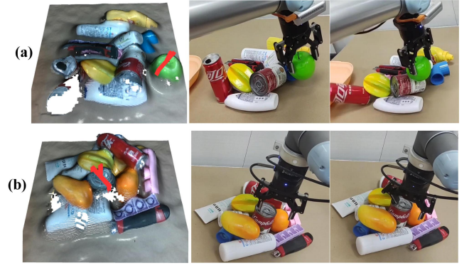
Fig.15. The ablation experiment for collision-free strategy, (a) represents the collision between the grasped target and the other target, (b) represents the collision between the gripper and the around target during the robot movement.
