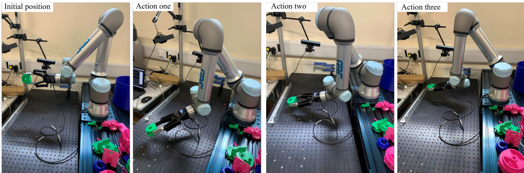
Figure 8. The experiment of UR5e: First, the initial position is set, then three target points are randomly assigned within the workspace, the target points are input to the PMP, and finally the PMP drive the robot to move from the initial position to the target sequentially.
