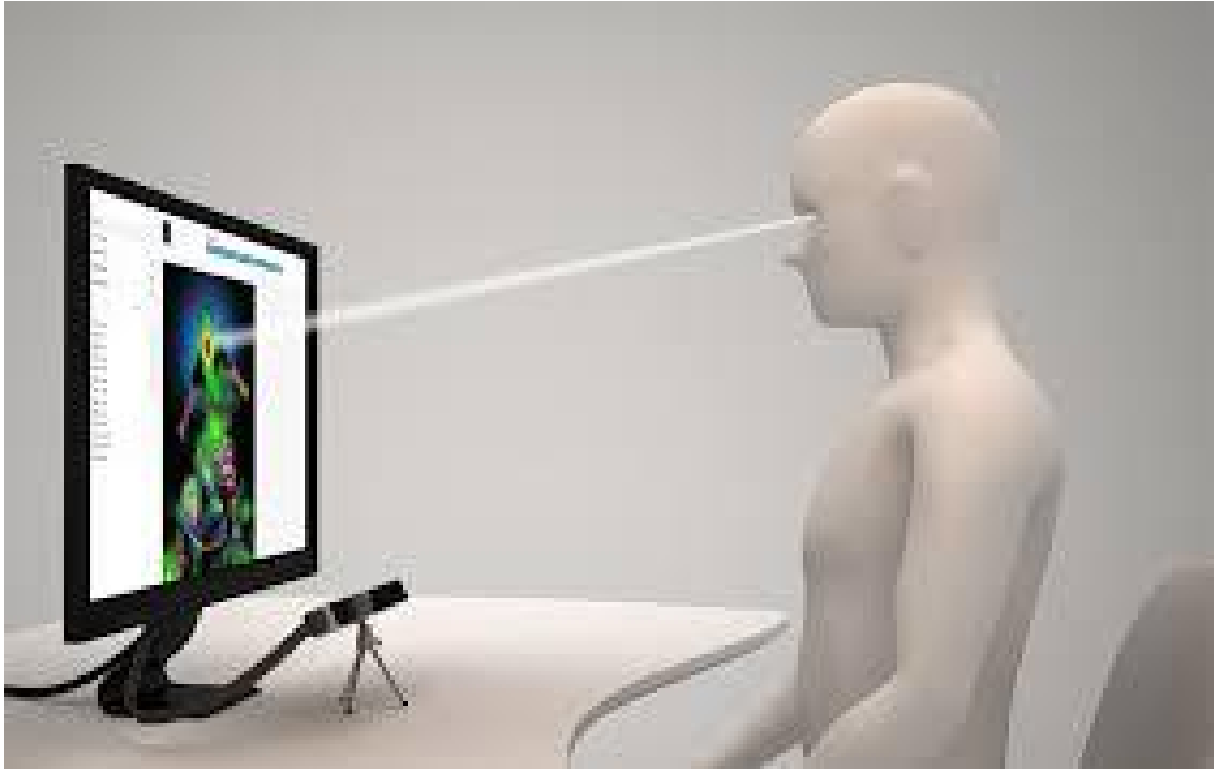
Figure 3.2: Collecting pupil data using an eye tracker [378].
