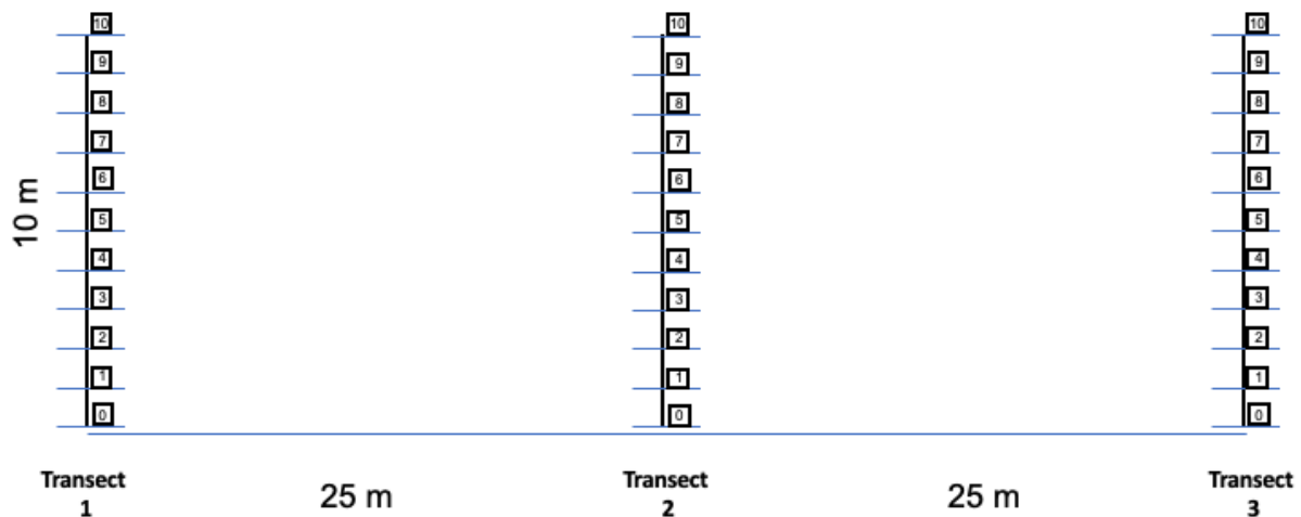
Figure 2.1. Transect placement for seagrass biometric measurements, adapted from the Seagrass Watch protocol (McKenzie, 2003).
