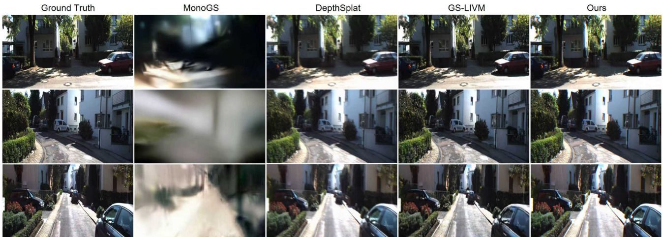
Fig. 5: Rendering on KITTI road scenes. Each row shows one representative frame. Columns (left to right) are Ground truth, MonoGS, DepthSplat, GS-LIVM, and MOGS. Our method reconstructs sharper thin structures, preserves depth discontinuities at boundaries, and suppresses long range floaters.
