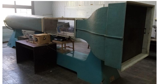
Figure 12: The wind tunnel which is used in the experimental setup.
