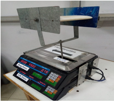
Figure 15: Lift and drag force measuring instrument.
