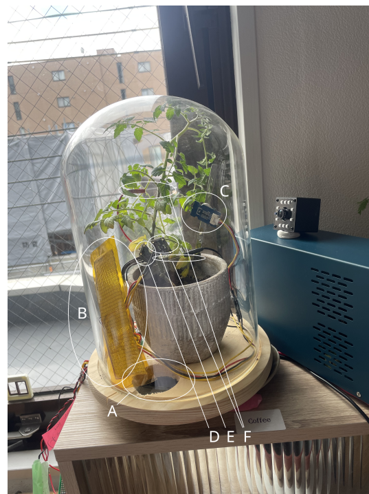
Figure 1. Annotated experimental setup. (A) Fan to flux fresh air. (B) Heating element providing controlled thermal perturbations. (C) SGP30 gas sensor measuring eCO 2 and total volatile organic compounds (TVOC). (D) LTR303 light and infrared sensor positioned at base height. (E) HDC302 temperature and humidity sensor located near the plant stem at mid-height. (F) Differential electrodes inserted into plant tissue for extracellular bioelectrical recordings (live electrode near canopy, reference electrode basally).
