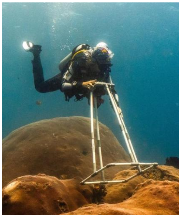
Figure B.1. A diver using a custom-built PVC frame (0.5 × 0.5 m) with a mounted Olympus TG6 camera to capture benthic images and assess the occurrence of the invasive coral-killing sponge Haliclona (Chalinula) nematifera . The structure, designed to withstand the strong currents and challenging conditions of the area, ensures that the entire quadrat area is included in each photo. Photo credit: Pedro Medeiros.
