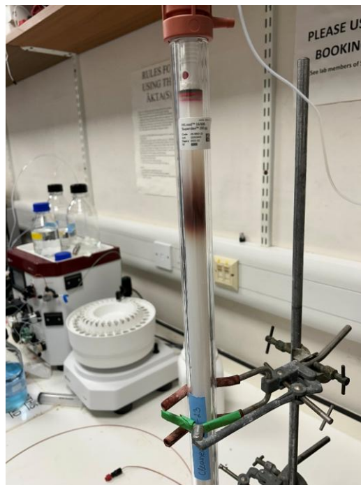
FIGURE 2.8 Image of the S200 size exclusion column running with loaded OleT JE . The major elution peak is at ~75 ml and is consistent with monomeric species with fractions of this peak being pooled and concentrated for experimentation.
