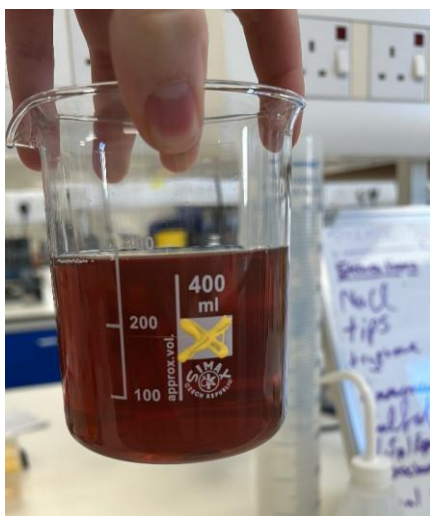
FIGURE 2.4 Images of clarified lysate. The left image was taken after cells were grown overnight, harvested and lysed using an Emulsiflex-C5, and then centrifuged to separate OleT JE from lysed cells before binding to a Ni-NTA column, as described in the experimental section
