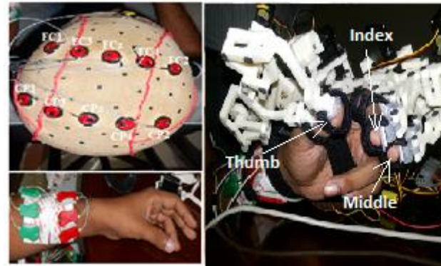
Fig.3 The EEG and EMG electrode placements(Left) and The Three Finger Exoskeleton mounted on subject's hand(Right).
