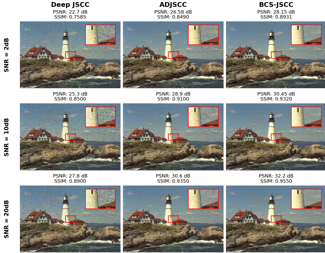
Figure 3.9: Example of reconstructed image produced by the proposed BCS-JSCC and the baseline methods with compression ratio of 1/6, \text{SNR}_{\text{train}} of 1 dB and \text{SNR}_{\text{test}} values of 2, 10 and 20 dB
