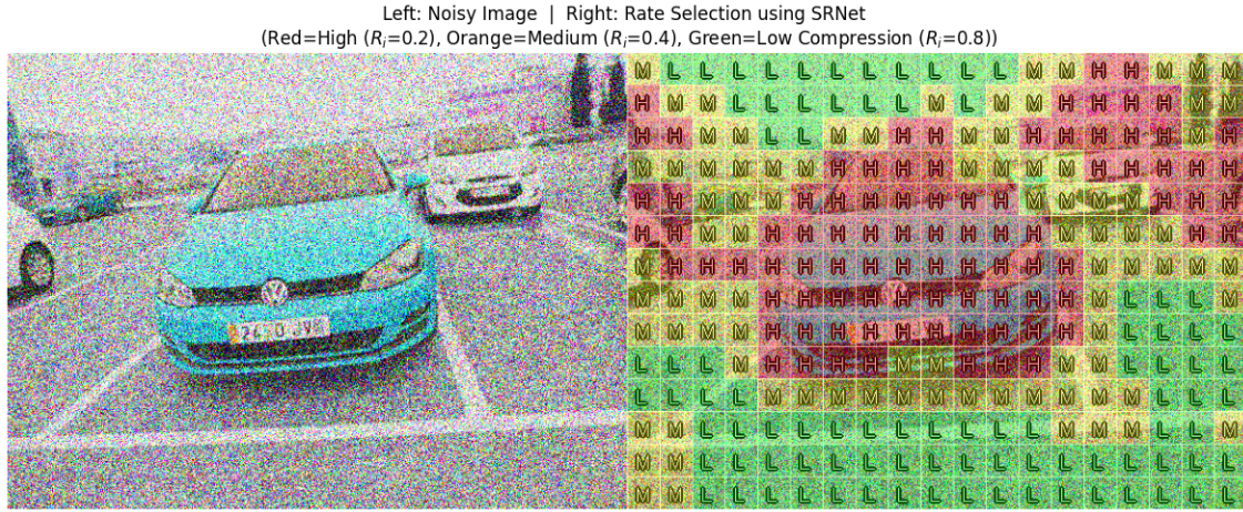
Figure 5.11: Block-wise sampling rate selection for license plate detection at low SNR. Red denotes high sampling density, orange medium, and green low.
