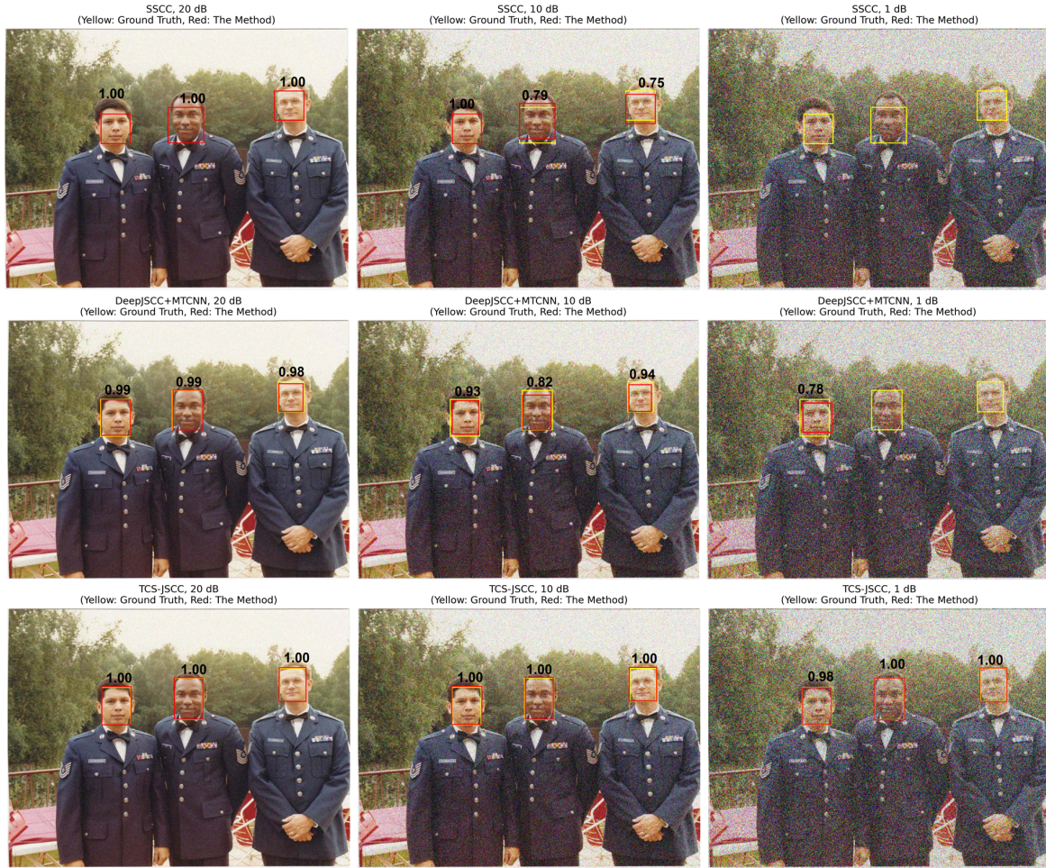
Figure 5.8: Visual comparison of detection outputs for SSCC, Deep JSCC+MTCNN, and TCS-JSCC at SNR levels of 20 dB, 10 dB, and 1 dB. Yellow boxes indicate ground truth, while red boxes show the detection results produced by each method. The overplotted numbers represent the detection confidence score.
