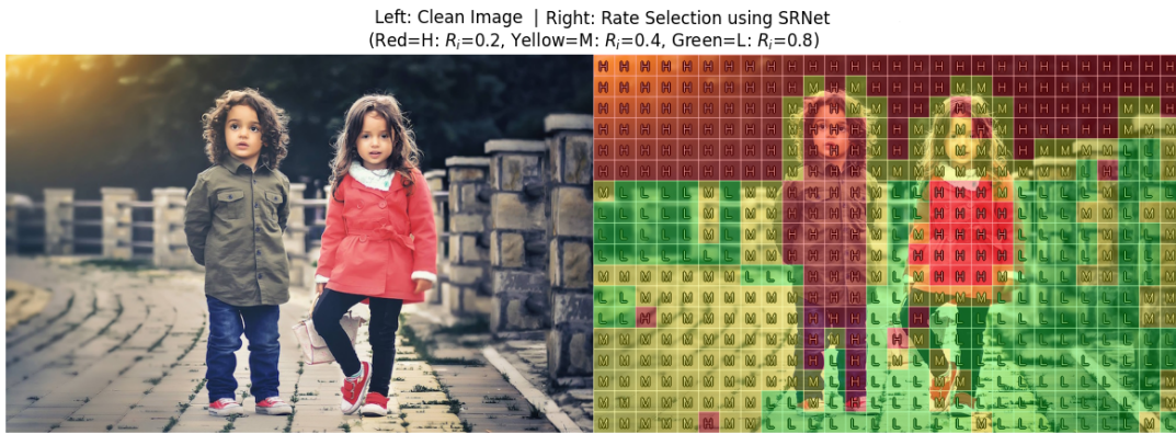
Figure 5.7: Illustrative SRNet block-wise sampling rate selection at SNR = 1 dB. Left: clean image. Right: per-block sampling rate map selected from \mathcal{R} = \{0.2, 0.4, 0.8\} .
