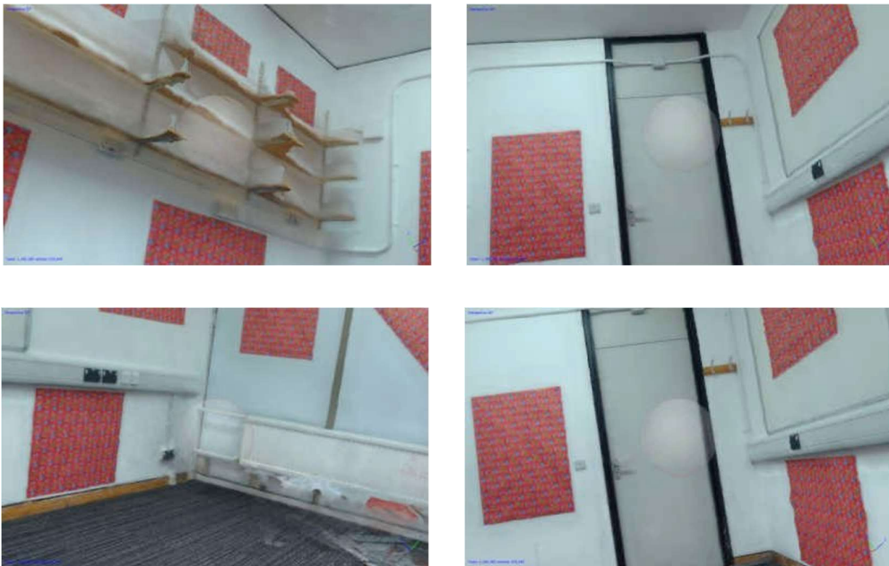
Figure 21- Reconstruction from a 5-megapixel dataset (540 images). Dense cloud density falls to approximately 140,000 points, a 25% reduction against the 8-megapixel baseline. The four panels show the resulting geometric artefacts, warped boundaries and surface irregularities, demonstrating that 5 megapixels falls below the threshold required for structural coherence.
