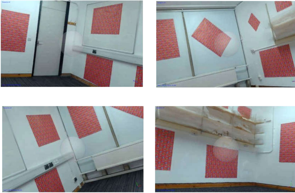
Figure 18- Reconstruction of the room following application of patterned surface texture, from 180 images. Alignment success rises from below 30% to above 95%, and dense cloud density approximately doubles relative to the untextured condition, identifying surface texture rather than image volume as the governing variable.
